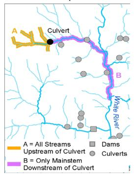
Figure 2: Culvert Stream Mile Delineation
